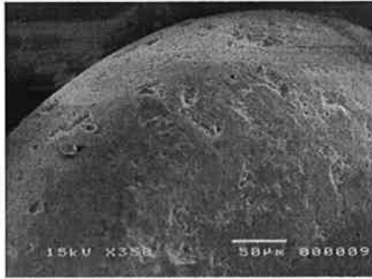
Figure 1.1 Scanning Electron Micrograph of sand media after 8 months installation in a pilot scale roughing filter. Biofilm growth is restricted to the pitted areas presumably due to protection from shear during filtration and from abrasion during washing.
