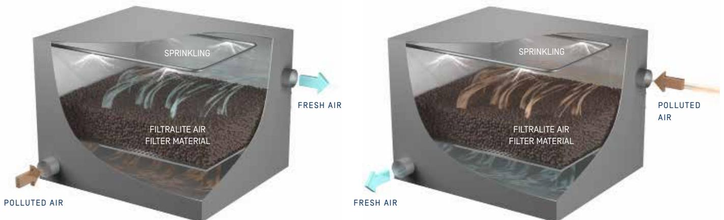
**Upstream system.** Polluted air is pushed upwards through the filter while sprinkling water drip downwards.
