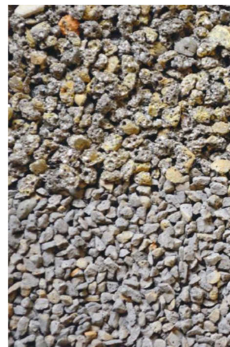
MONO-MULTI: Filtralite at work, note its porous nature and distinct layers
