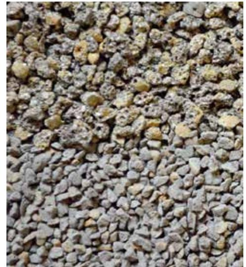
MONO-MULTI: Filtralite at work, note its porous nature and distinct layers
