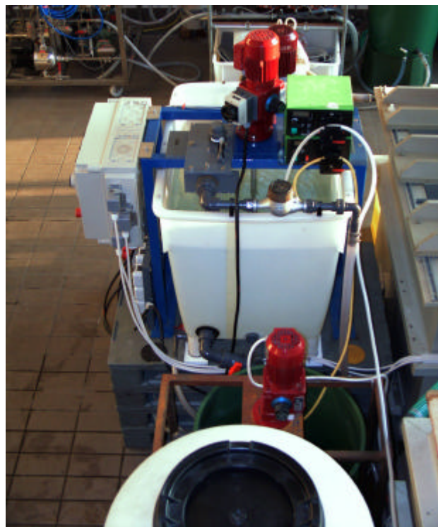
Fig. 2-2: Wastewater tank (in foreground, white with black cap), clay suspension (middle, dark green, with red stirrer) and mixing basin (white, with two peristaltic dosing pumps (green) on top and stirrer (red))
