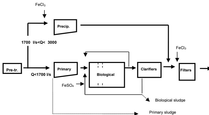
Figure 1 Flowchart Bekkelaget WWTP, water processes
