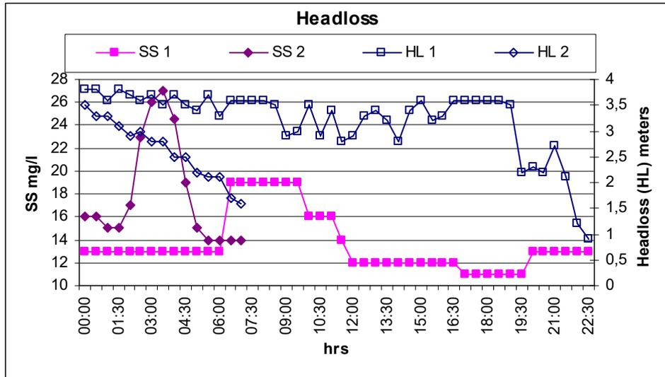
Figure 4. Headloss curves for a filter under different conditions. SS – mg/l HL – m
