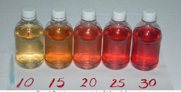
Figure 1: Potassium permanganate (mg/L) demand of raw water
