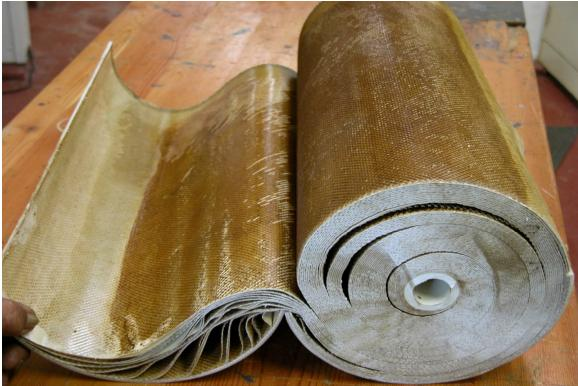
Figure 2: Picture of biofouled membrane following pre-treatment using manganese greensand.
