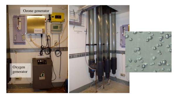
Figure 8. The generators, the six ozonation columns and ozone bubbles.
