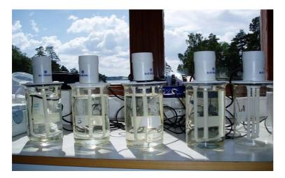
Figure 11. The jar test equipment.
